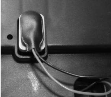
9-V-block battery for emergency lowering
