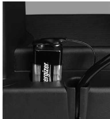
9-V-block battery for the emergency lowering
