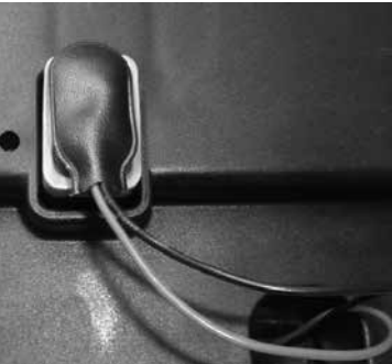
9-V-bloc battery for emergency lowering
